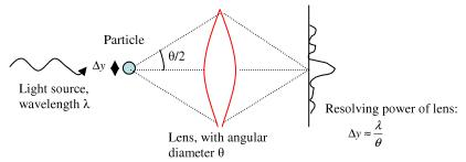
Photons transfer momentum to the particle when they scatter.
